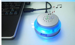
USB-Speaker-HUB 3 Ports USB Hub 2.0 & Mini Speaker With 6 blue LEDs With USB cable and Audio cable Size 60x60x35mm
